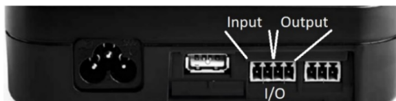
Figure 21: DCONNECT BOX2 INPUT / OUTPUT
