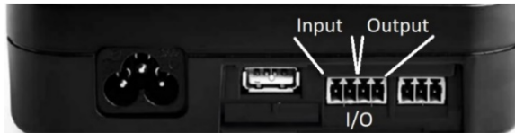
Figura 21: INPUT / OUTPUT DCONNECT BOX2
