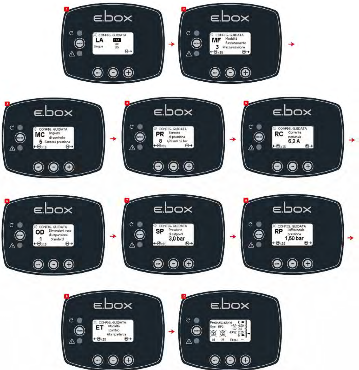
Figure 12: Configuration with a pressure sensor
