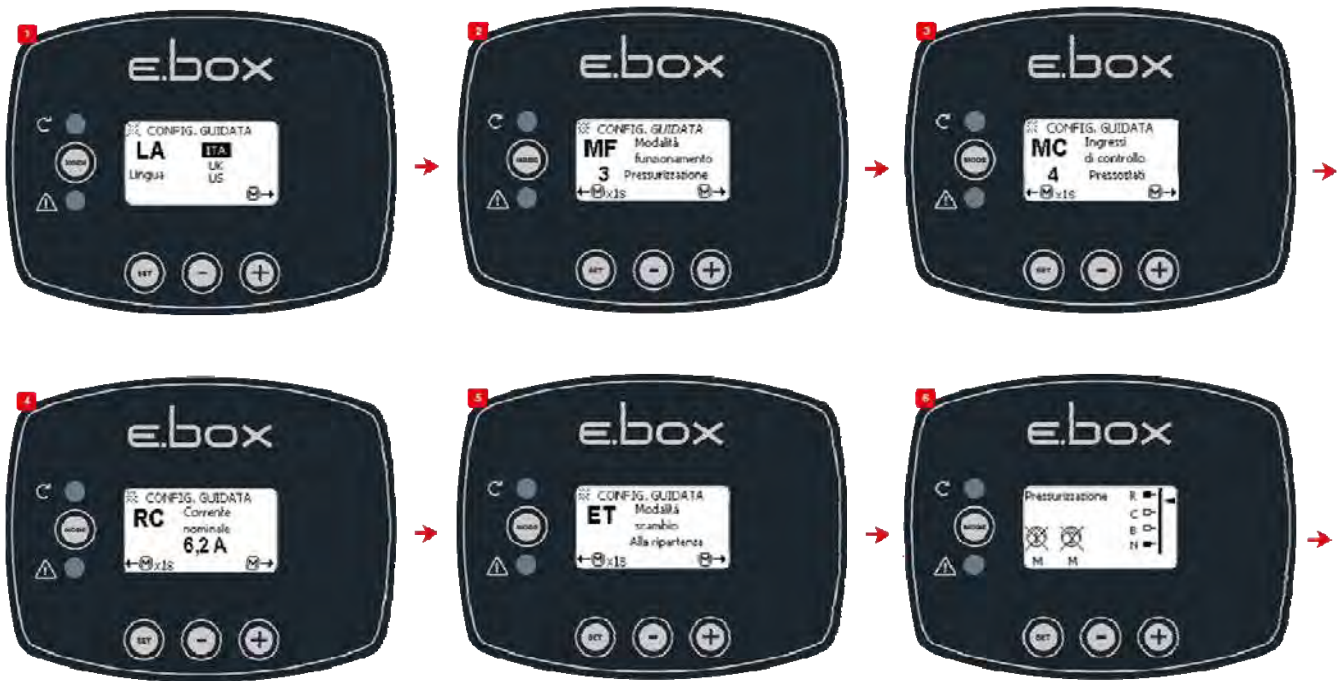
Figure 13: Configuration with pressure switches
