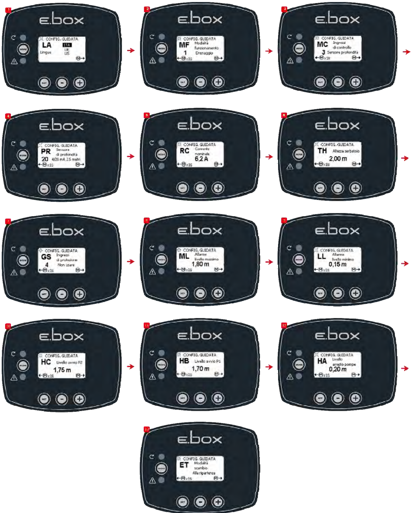
Figure 38: Configuration with only a depth sensor
